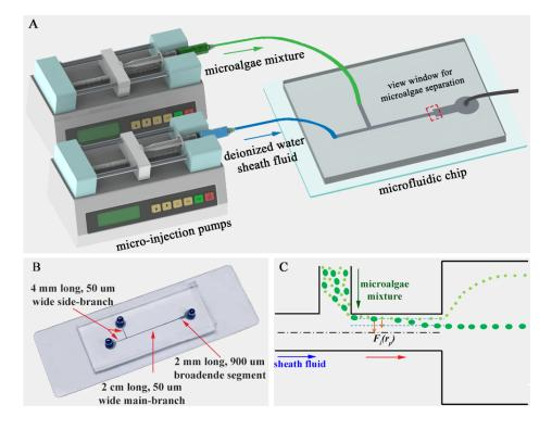
Figure 1. The diagram of the microalgae separation system (A)and the microfluidic chip (B) designed for the experiment. The chip is filled with black ink for clarity. The schematic diagram of the microalgae separation via iPFF is drawn not scale (C). The inertial lift forces are indicated by  $F_i$ . The solid arrows indicate the flow direction in the sheath flow (blue), microalgae mixture (green) and main channel (red).
