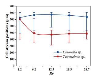
Figure 3. The effects of the fluid inertia (*Re*) on the stream positions for the *Chlorella* sp. (blue circle) and *Tetraselmis* sp. (red square). The bottom sidewall of the channel expansion was used as the reference point (0  $\mu$ m). Error bars were included for both cells in Figure 2 to cover the span of each cell stream. Confidence interval of the graph is 95%.
