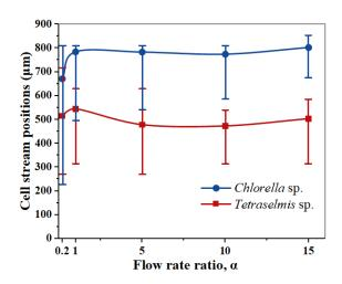
Figure 5. The effects of the flow rate ratio ( $\alpha$ ) on the stream positions for the *Chlorella* sp. (blue circle) and *Tetraselmis* sp. (red square). The bottom sidewall of the channel expansion was used as the reference point (0 µm).
